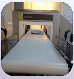
Combo Checkweigher With Metal Detector
